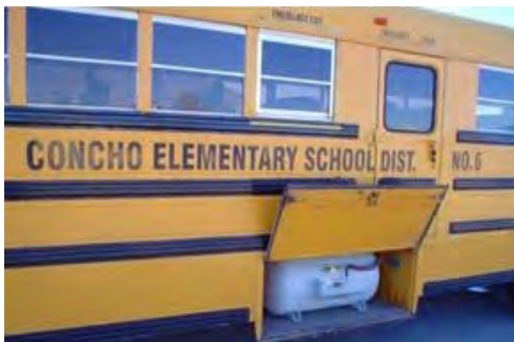
Figure 8: Arizona school bus converted into a bi-fuel propane vehicle. (56)
