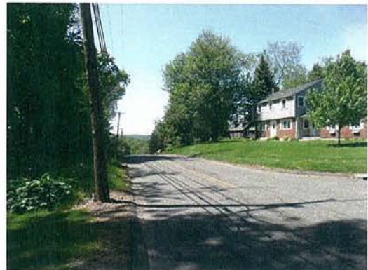
Steep slope on Allen Avenue limits intersection sight distance on Hourigan Street (West) looking northwest
