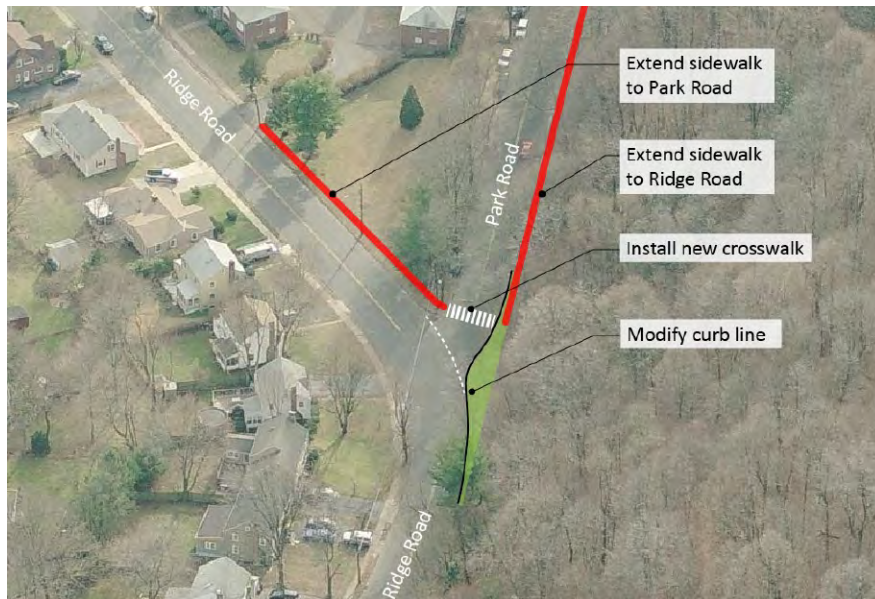
5. Realign curb at Ridge Road. Install curb ramps and crosswalk. Extend existing sidewalk on Park Road to Ridge Road.
