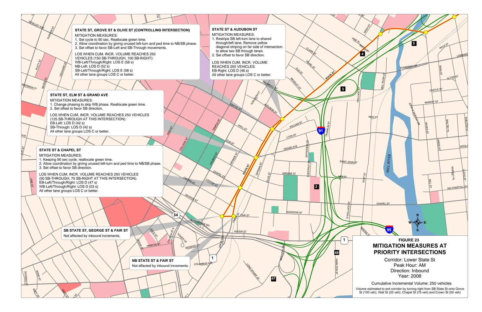
approach at Audubon Street to shared through/left, and remove the yellow diagonal striping in the southbound lanes south of Audubon Street to provide two lanes for through traffic.
