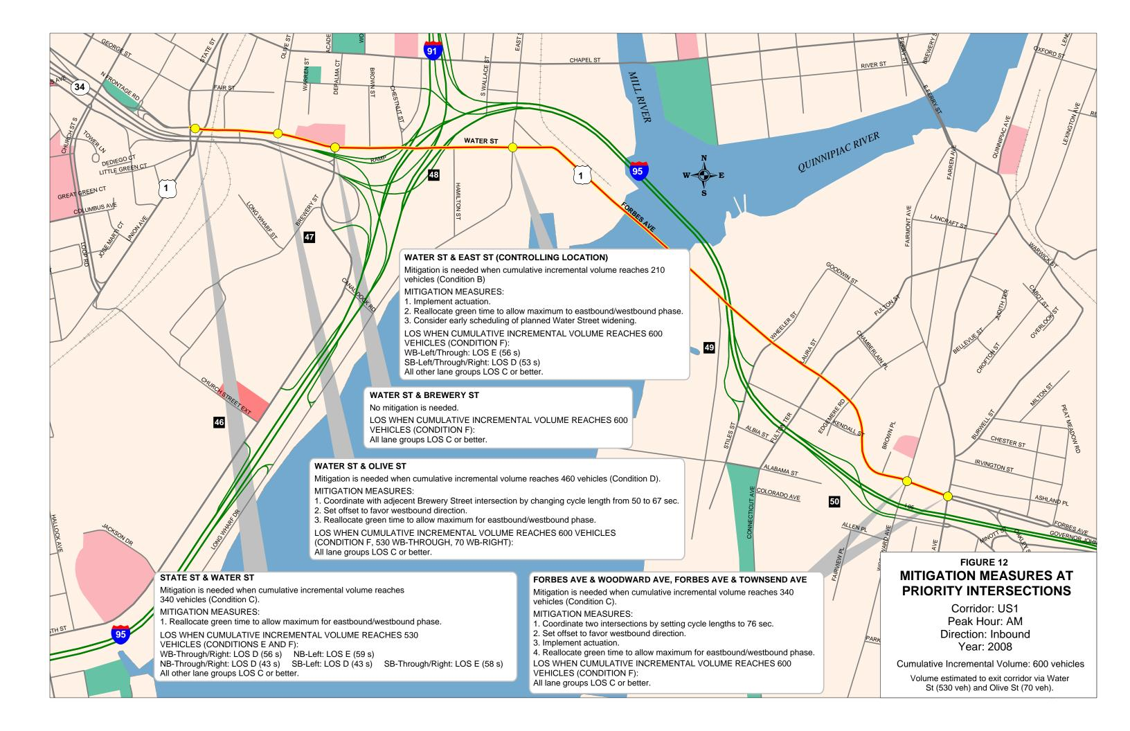
cycle. Unused time was given to the eastbound-westbound phase. Also, using the same 104 second cycle length, green time was reallocated so that the minor movements operated near the threshold, thus allowing maximum green time for additional westbound traffic.
