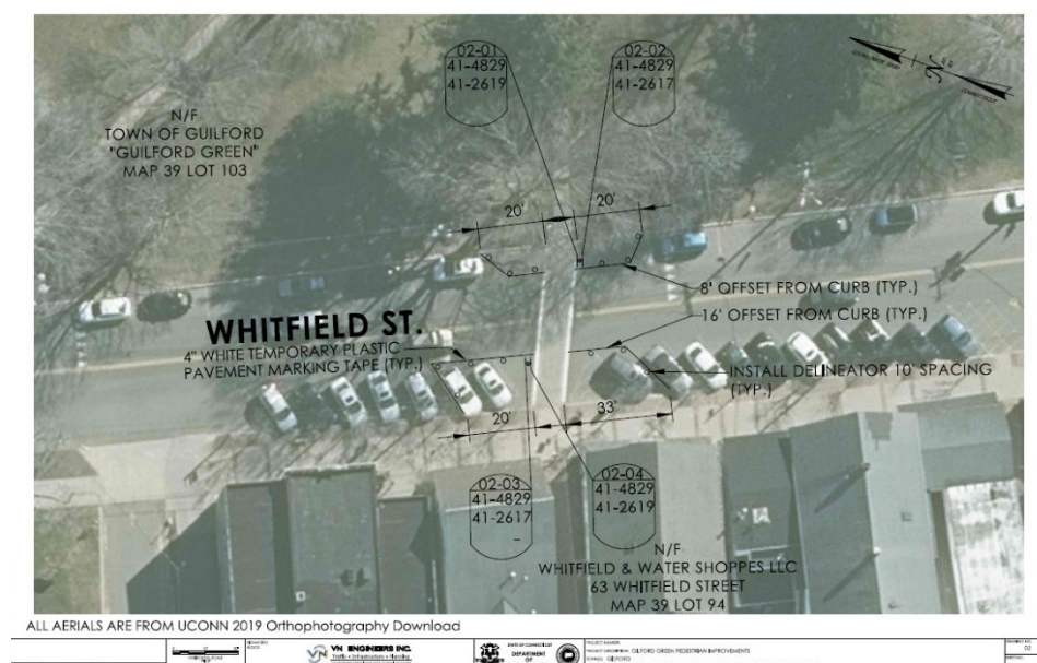
Figure 34 63 Whitfield Street Temporary Curb Extension Diagram
