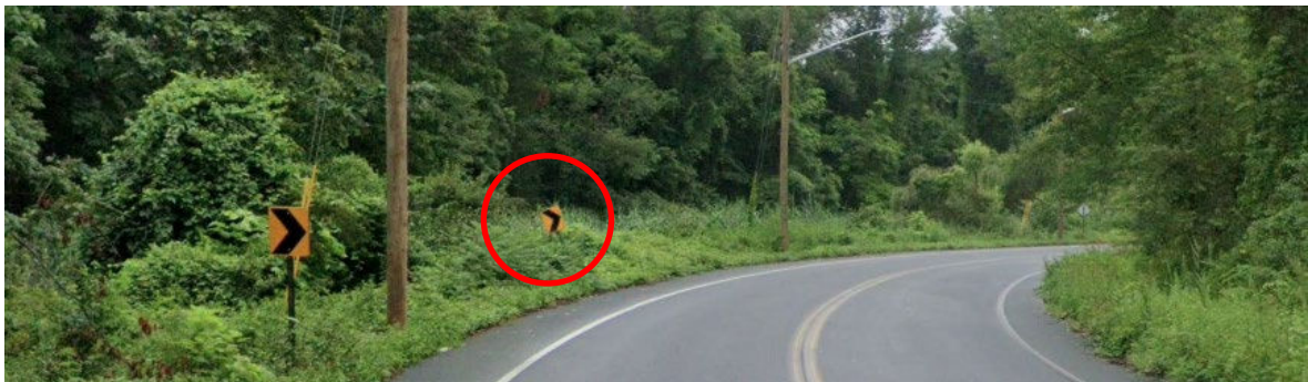
Figure 14 Vegetative Removal or Pruning Location 3 – Chevron Sign in Southbound Direction
