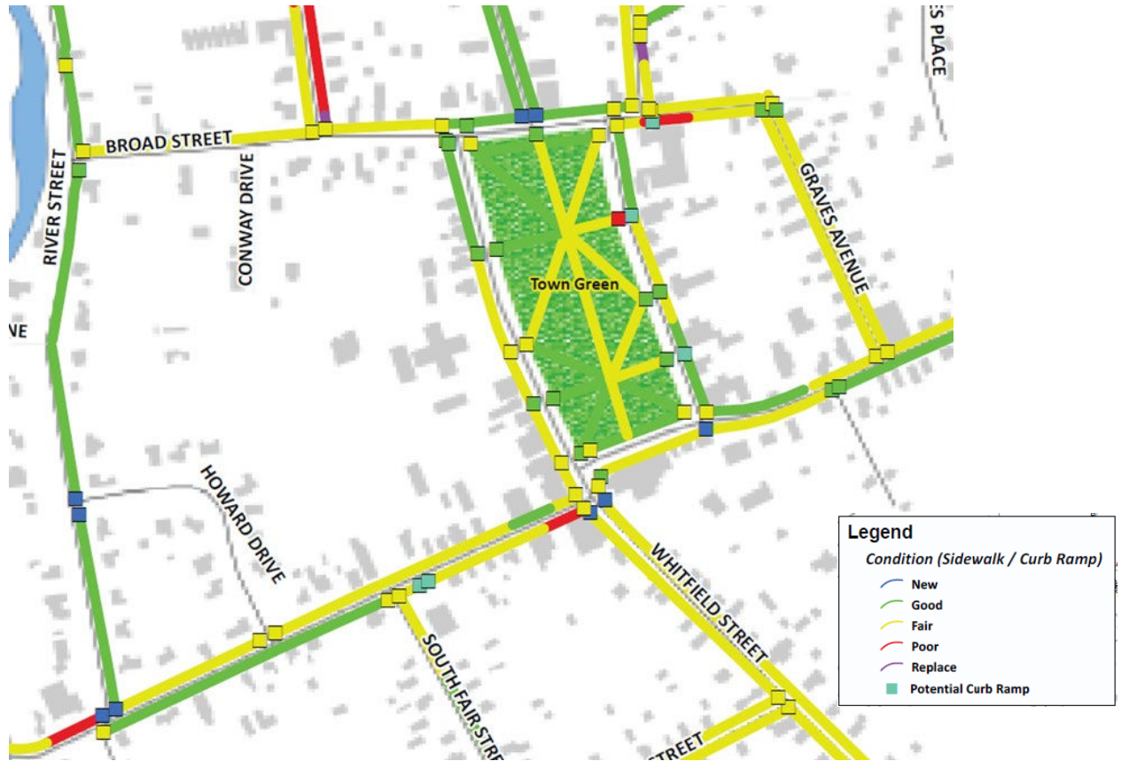
Figure 10 Curb Ramp and Sidewalks Conditions Around Guilford Green
