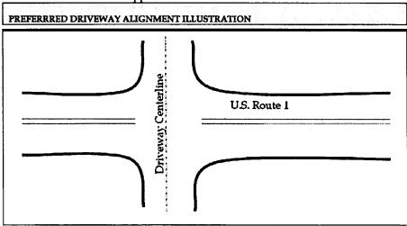
(2) If such alignment is not feasible, new driveways shall be offset from existing driveways or streets a minimum of 250 feet along arterials or thoroughfares, and 150 feet along collector streets.
