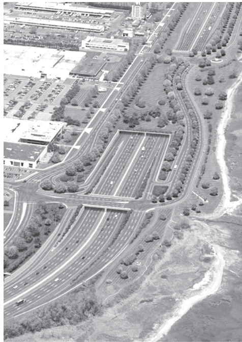
Figure 8: I-95 Options at Long Wharf. Early design suggests that an at-grade facility is likely to prove necessary given high costs associated with a depressed section and poor experience with elevated facilities. Illustrations and freeway cost courtesy of the Connecticut Department of Transportation and Parsons Brinckerhoff appearing in Parsons Brinckerhoff Quade & Douglas, Preliminary Engineering Study, New Haven Harbor Access , prepared for ConnDOT (Glastonbury: Parsons, 2002). Plan proposals target another $86 million for local roadway and harborside access improvements.
